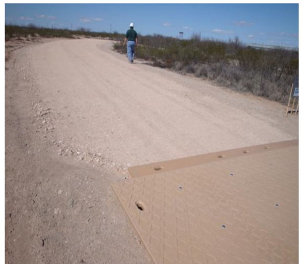
Testing of composite mats and recycled drill cuttings as road materials. Recycled drill cuttings supplied by Scott Environmental Services. Composite mats supplied by
